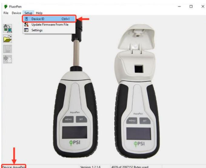
Fig. 18 Connecting AquaPen to software.
