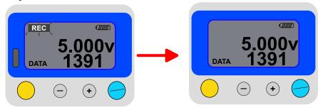
Press the record/stop button for 2 seconds or more, and stop is completed when "REC" disappears after blinking.
