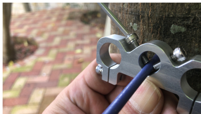
9. Please tighten bracket screw from both side.
