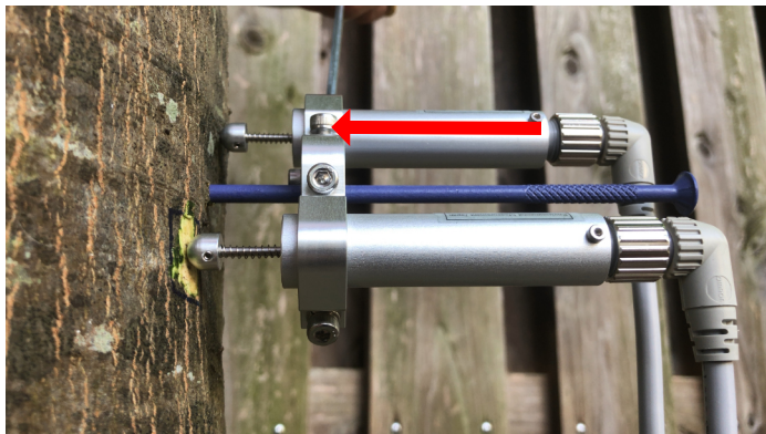
14. Push the other LM toward tree and tighten LM by using screw at bottom of bracket.
