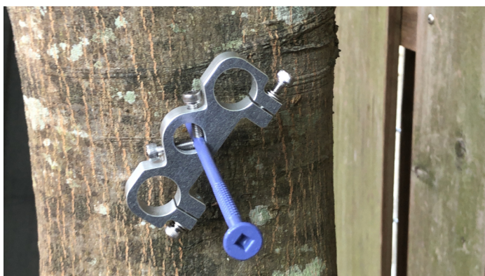
10. Since this tree is thin; thus, the xylem may destroyed when drill the tree so set Installed bracket diagonally.
