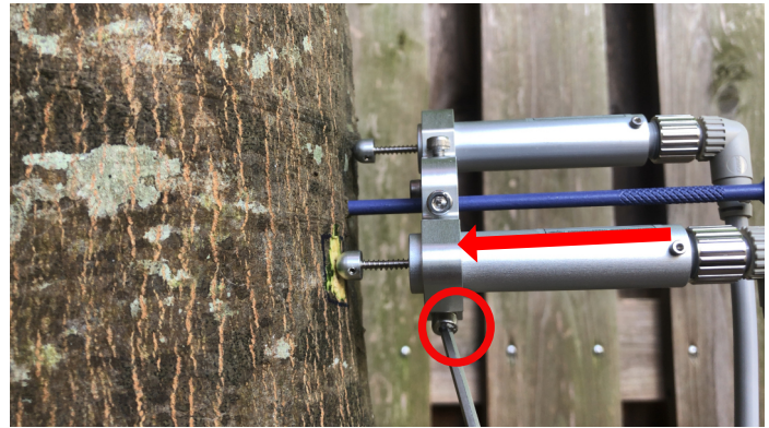
13. Push the LM and tighten LM by using screw at bottom of bracket. This picture shows the front LM is pushed toward tree.
