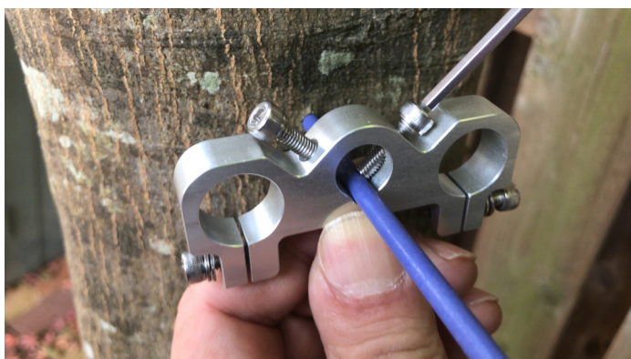
8. Set the MIJ-02 Bracket to the long screw.
