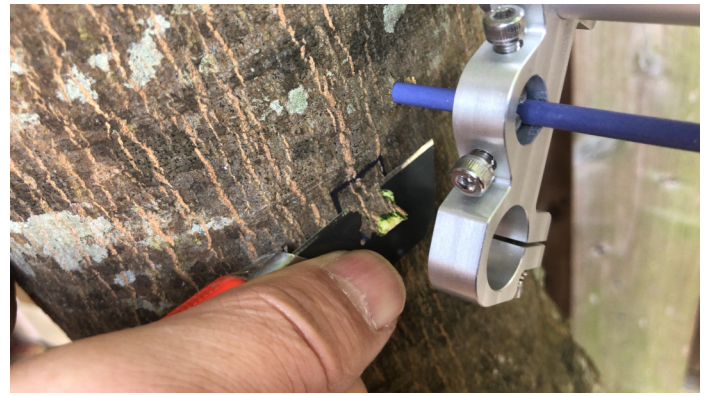
11. Remove the LM for shaving bark.
