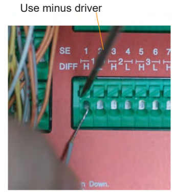
Figure3. Connecting the sensor
