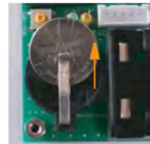
How to remove the backup battery
