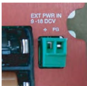
External power input terminal
