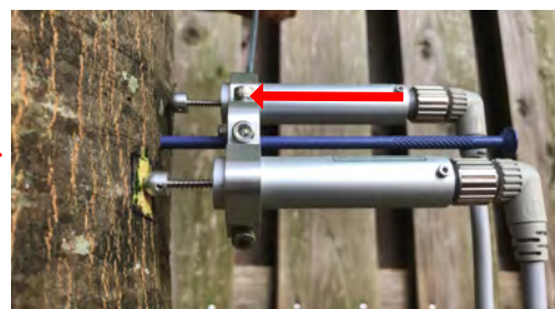
14. Push the other LM toward tree and tighten LM by using screw at bottom of braket.
