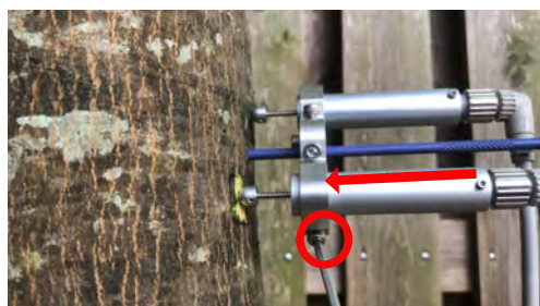
13. Push the LM and tighten LM by using screw at bottom of braket. This picture shows the front LM is pushed toward tree.
