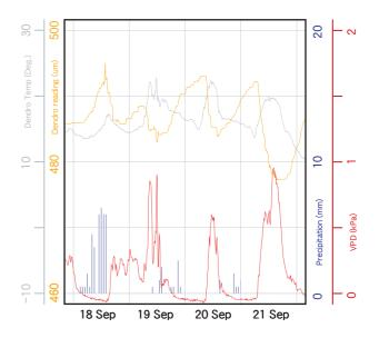
MIJ-02 LM Type2 can measure with less than 0.1um resolution and also be able to analyze process of sapwood shrinks occur from sapflow and relation with sapwood pressure potential. As annual changes, individual carbon fixation and production from individual live tree will be the direct index which can lead estimation of whole canopy value.
